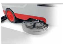
The brush pressure can be adjusted up to 100 Kg for hard cleaning
